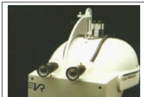
Gambar 2.6 Contoh *Opaque HMD*, Courtesy Jannick Rolland, Frank Biocca, dan UNC Chapel Hill *Dept. of Computer Science*. Gambar dari Alex Treml. (Azuma 1997)
