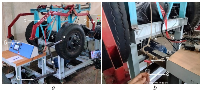
Fig. 1. Rotational brake test rig: a – subsystem configuration for evaluating hydraulic brake failure and secondary safety brake performance; b – leakage process mechanism
