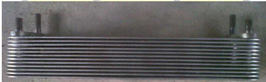
GAMBAR 3 HEAT EXCHANGER EVAPORATOR
