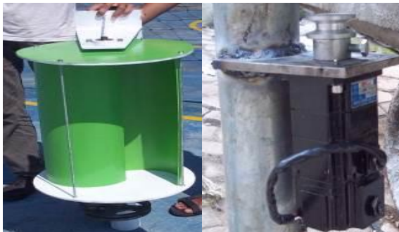
Fig. 7 Savonius turbine & Generator 200 W
