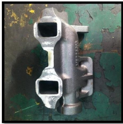
Gambar 4.6. Casting Exhaust Manifold
