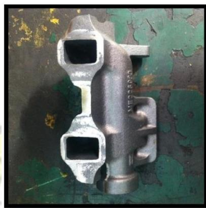
Gambar 4.6. Casting Exhaust Manifold
