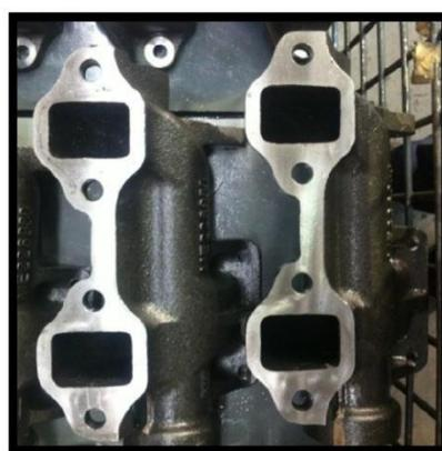
Gambar 4.5. Exhaust Manifold Finish Produk
