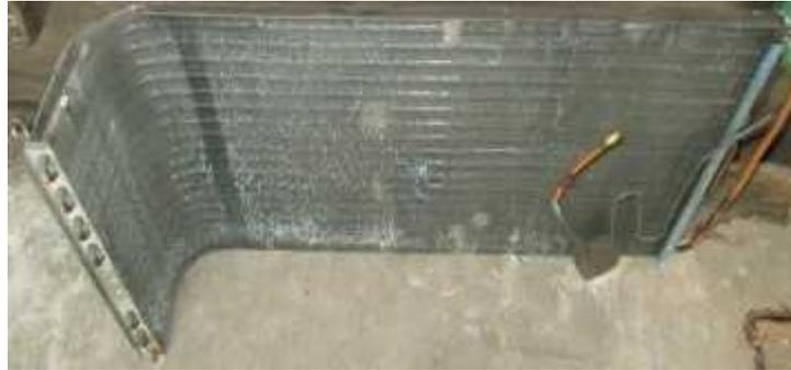
**Gambar 2.2.1.3 Kondensator**
