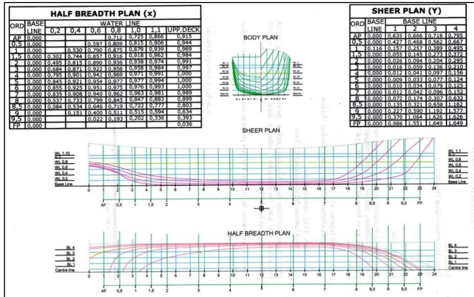
Figure 2: The Longline vessels lines plan
