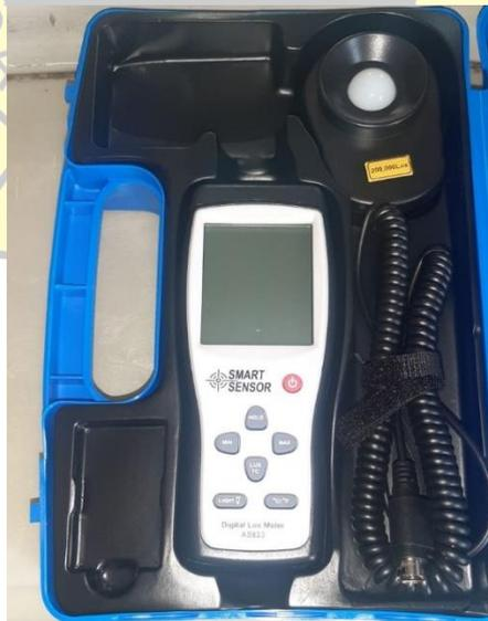
**Gambar 2. 1** Alat Ukur *Lux meter*
