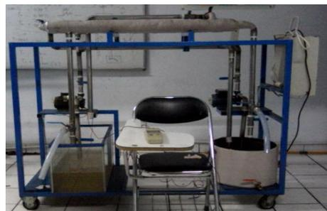
**Gambar 3.2** Alat heat exchanger
