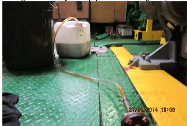
**Figure 6.** Overflow from M/E to daily tank
