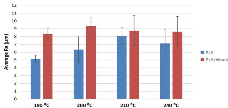
**Figure 4.** Roughness comparison graph of PLA and PLA/Wood composite at each temperature
