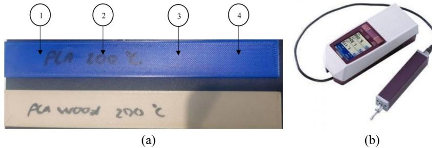
**Figure 2.** (a) Surface roughness test specimens and measurement areas, (b) Portable surface roughness tester Mitutoyo SJ-210
