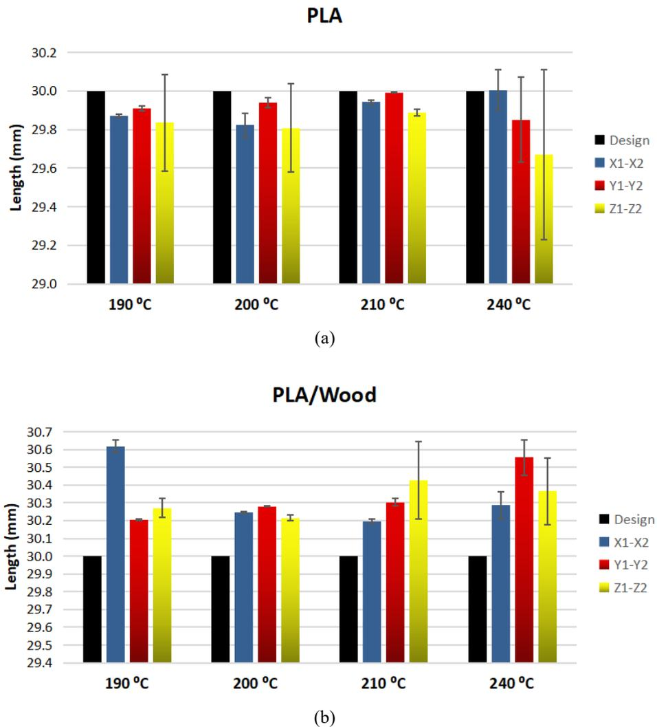
**Figure 6.** Graphical representation of dimensional accuracy test for (a) PLA, and (b) PLA/Wood composite samples
