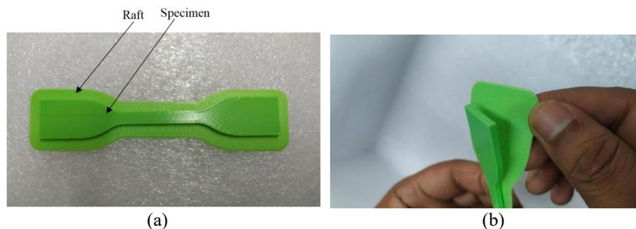
**Figure 5.** (a) Printed tensile specimen with a raft, (b) raft removal by hand
