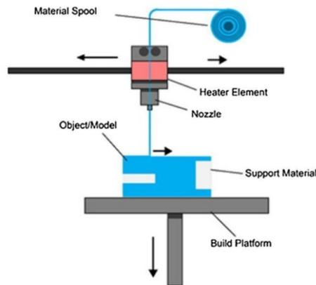
**Figure 1.** The principle of the Fused Deposition Modeling process [1]
