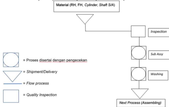
Gambar 3. Peta Proses Operasi Area Assembling Part F/G
