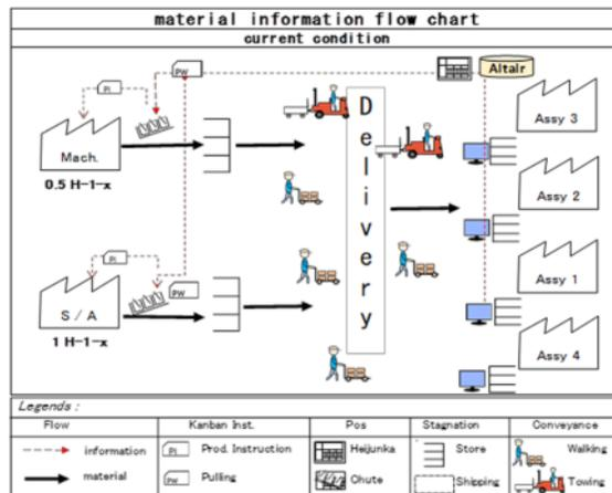
Gambar 4. MIFC Penanganan Manual Transfer Material
