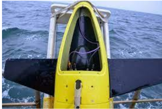
6 Gambar 2.6: Gambar Oil Bladder di dalam Underwater Glider
