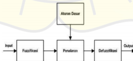
Gambar 3.2 Blok diagram logika fuzzy (Sumber: NUG, 2010)
