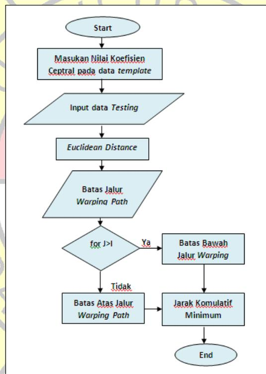
Gambar 2. Flowchart proses testing Dynamic Time Warping
