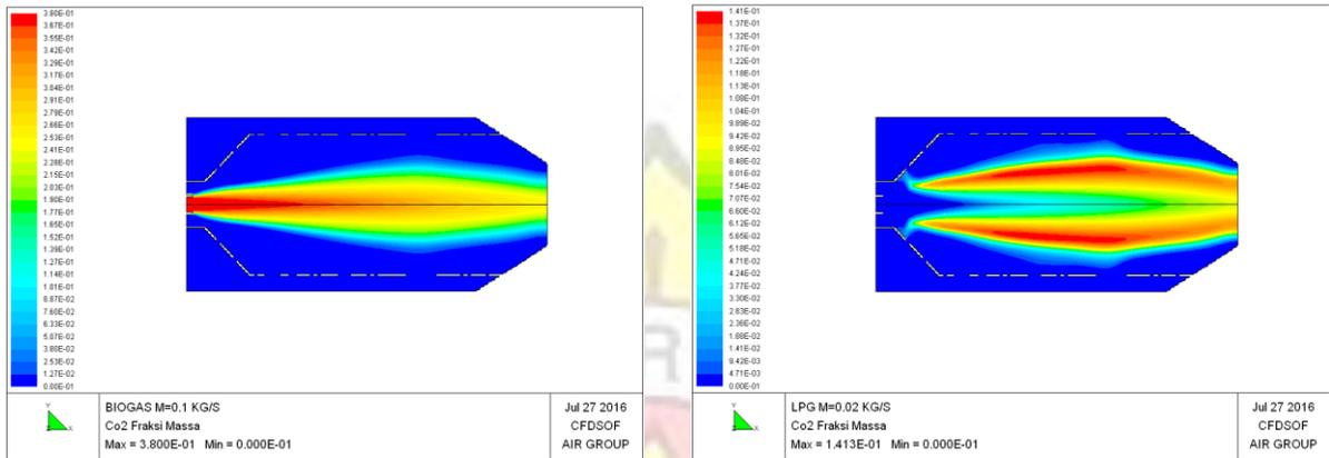
Gambar 6. Fraksi massa CO<sub>2</sub> (a) biogas, (b) LPG.
