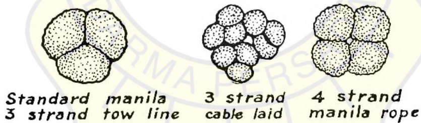
Gambar 4. Tipe Pintalan – pintalan Serat tali ( Tugs, Towboats, dan Towing Edward M. Brady 1979 hal 69 )
