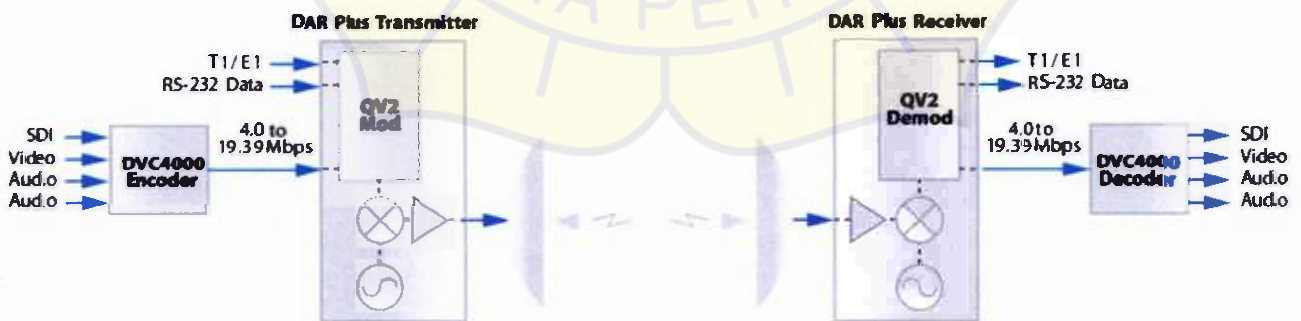
Figure 1 – Simplex Configuration showing DVC4000 Encoder & Decoder used with QV2 Modulator and Demodulator
