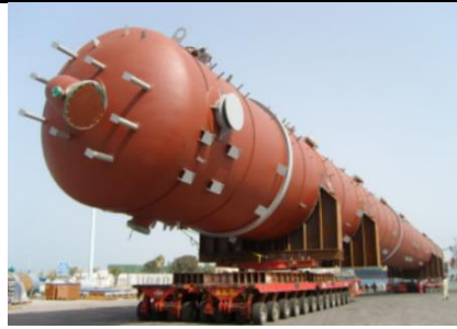
Gambar 2. 16 Ro-Ro using Modular trailers
