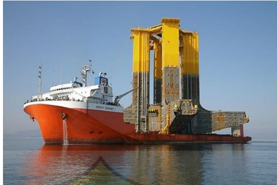
Gambar 2. 7 SSHV membawa Offshore Platform
