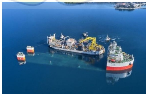
Gambar 2. 17 Float On Semi Submersible Heavy Lift Vessel
