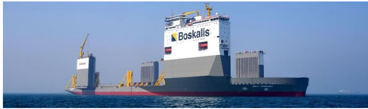
Gambar 2. 2 Semi Submersible Heavy Lift Vessel
