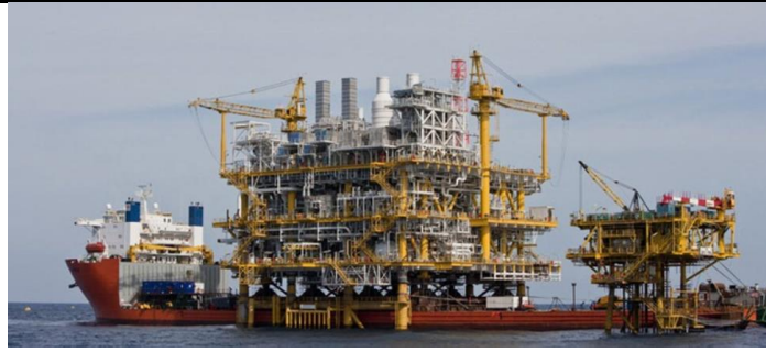
Gambar 2. 11 SSHV Dry Transport Oil Platform
