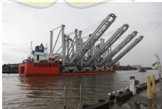
Gambar 2. 13 SSHV Dry Transport Container Cranes
