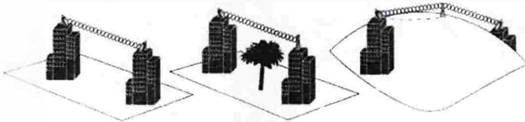
Figure 3. Crossing Great Distances with Cisco Aironet Bridge Antennas
