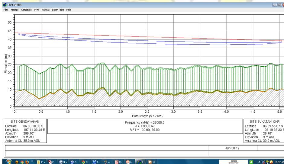
Gambar 4.2 Path Profile Microwave Link
