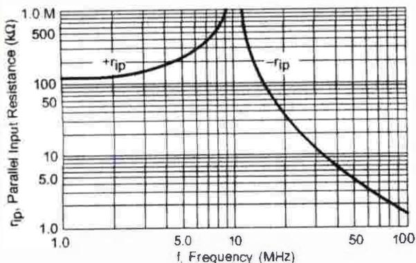
Figure 10. Signal-Port Parallel-Equivalent Input Resistance versus Frequency
