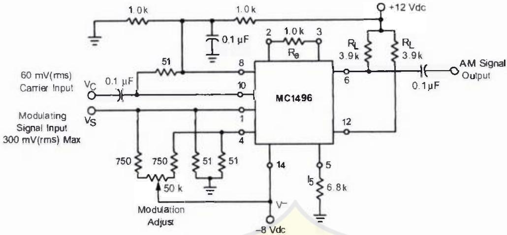
Figure 7. Amplitude Modulator
