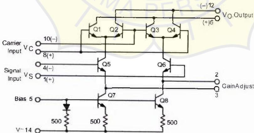
Figure 1. MC1496 Schematic
