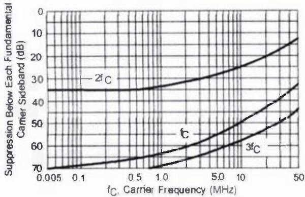
Figure 4. Balanced Modulator Carrier Suppression versus Frequency
