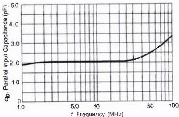
Figure 11. Signal-Port Parallel-Equivalent Input Capacitance versus Frequency
