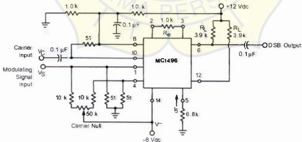
Figure 3. Balanced Modulator Circuit
