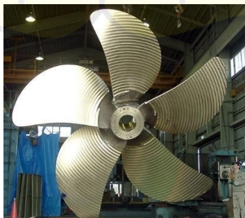
Gambar 2. 1 Fixed Pitch Propeller ( Sumber JURNAL TEKNIK ITS ).
