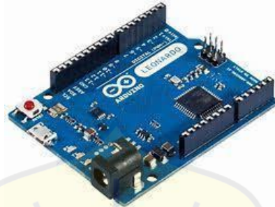
Gambar 2.6.2 Board Arduino Leonardo
