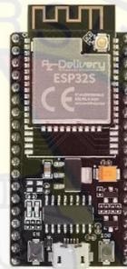
**Gambar 2.1** NodeMCU ESP32
