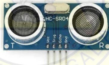
**Gambar 2.3** Sensor Ultrasonik hc-sr04
