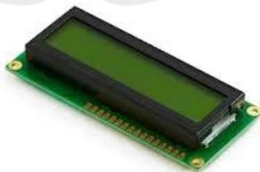
**Gambar 2.7** Liquid Crystal Display (LCD)
