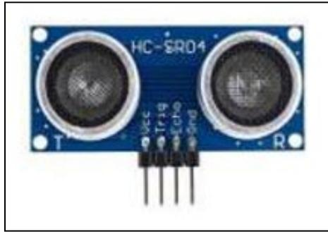
*Gambar 2. 5 Sensor Ultrasonik HC-SR04
