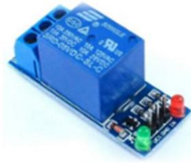
*Gambar 2. 7 Relay 1 Channel*
