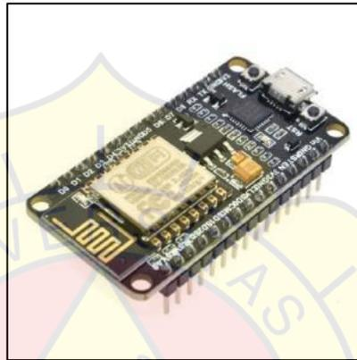
Gambar 2.1 NodeMCU ESP8266 (Efendi, 2019)
