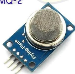
**Gambar 2. 7 Sensor Gas MQ-2**
