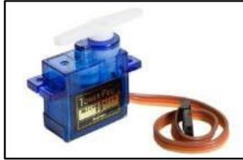
**Gambar 2.9** Servo motor
