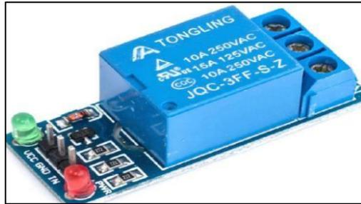
**Gambar 2. 9** Relay Module 1ch
