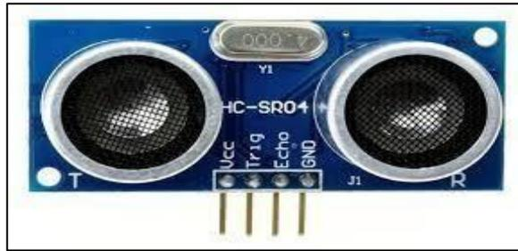
**Gambar 2.2 Sensor Ultrasonic** (Santoso, 2020)
