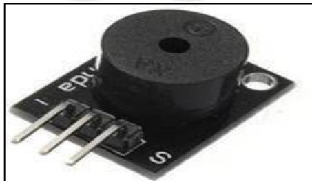
*Gambar 2. 4 Buzzer* (Ramady et al., 2020)
