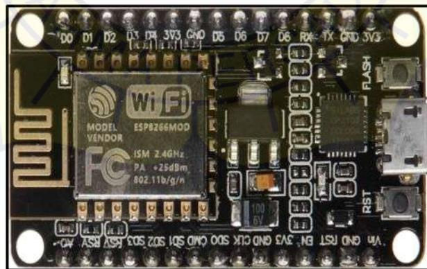
**Gambar 2. 1** NodeMCU V3 ESP8266
