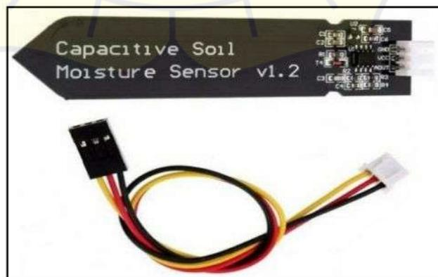
**Gambar 2. 2** Sensor Soil Moisture v1.2
