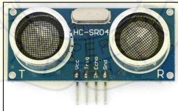
**Gambar 2. 3** Sensor Ultrasonik HC-SR04
