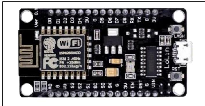
Gambar 2.1 *NodeMCU ESP8266* (Indra et al., 2021)
