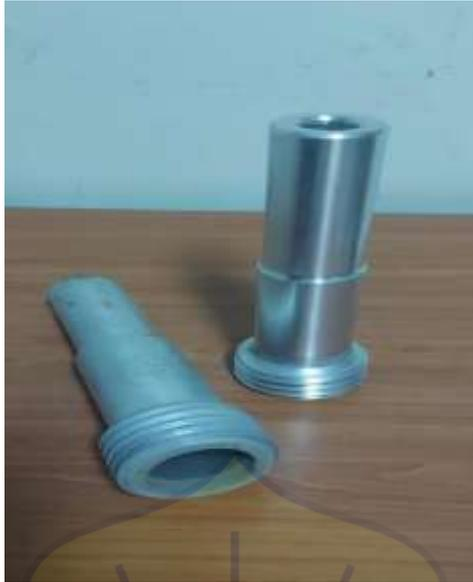
Gambar 2 17 – Sandblasting Nozzle No 7
