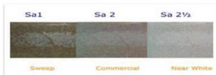
Gambar 2 14 – Sand Abrasive standard
